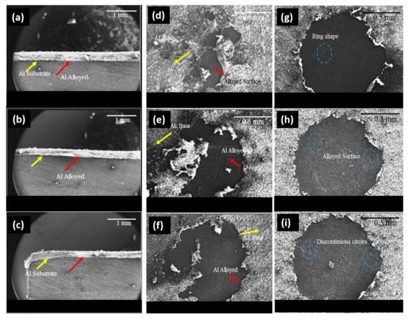
Fig. 2 SEM images showing cross-sectional views of the sample treated at different laser pulses: (a) 3, (b) 5, and (c) 7 pulses with a magnification of  $25 \times$ , and (d-f) the corresponding top-views of the sample with a magnification of  $70 \times$  (red arrow: Al substrate; yellow arrow: alloyed region). (q-i) Top-views of the sample treated at (q) 9, (h) 11, and (i) 13 pulses with a magnification of 70×.
