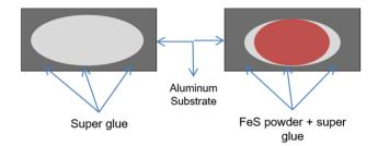
Configuration of the Fe-SiC coated aluminum substrate.
