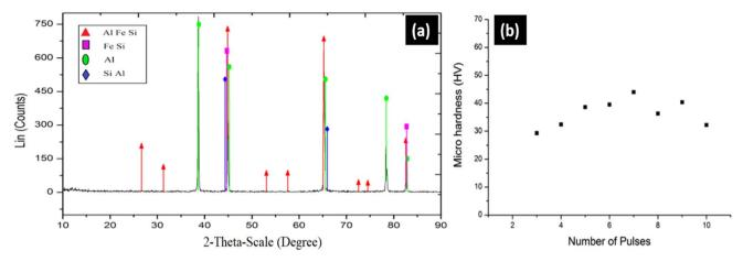
Fig. 4 (a) XRD analysis of the Al modified surface and (b) microhardness of the Fe-Si-C coated surfaces treated with different numbers of laser pulses.
