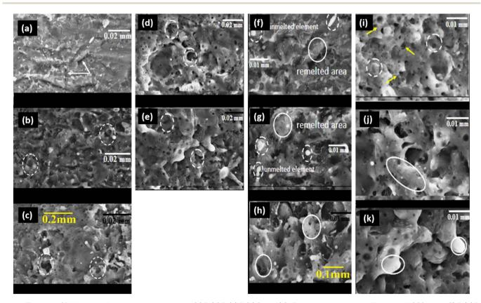
Fig. 3 Top-view SEM images of the samples treated with (a) 3, (b) 5, (c) 7, (d) 9, and (e) 13 laser pulses at a magnification of  $1000 \times$ , and (f) 3, (g) 5, (h) 7, (i) 9, (j) 11, and (k) 13 laser pulses at a magnification power of  $2000 \times$ .
