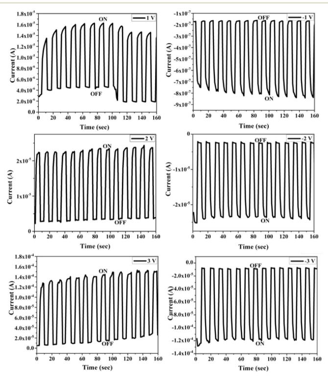
Bias voltage dependent relaxation response curves of the proposed MSM UVPD made of the Fe-SiC on aluminium layer.
