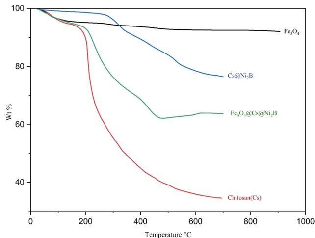
Fig. 4 TGA diagrams of chitosan (CS), Fe<sub>3</sub>O<sub>4</sub>, CS@Ni<sub>2</sub>B, and Fe<sub>3</sub>O<sub>4</sub>@CS@Ni<sub>2</sub>B.
