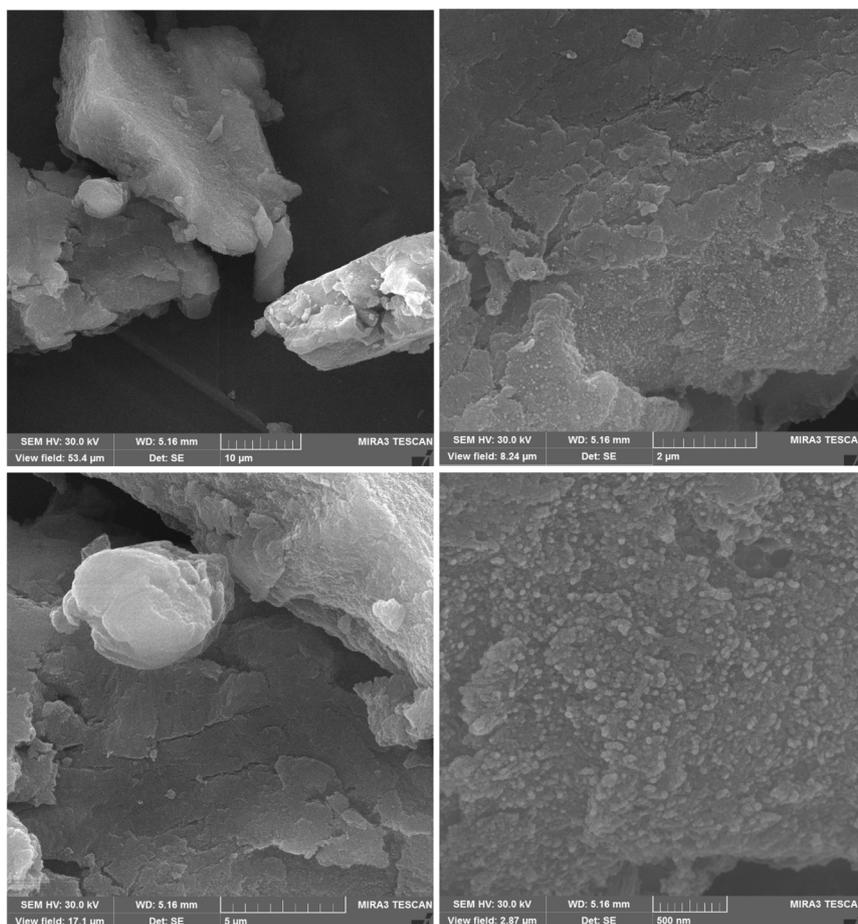
Fig. 7 FESEM image of the CS@Ni<sub>2</sub>B nanocomposite.
