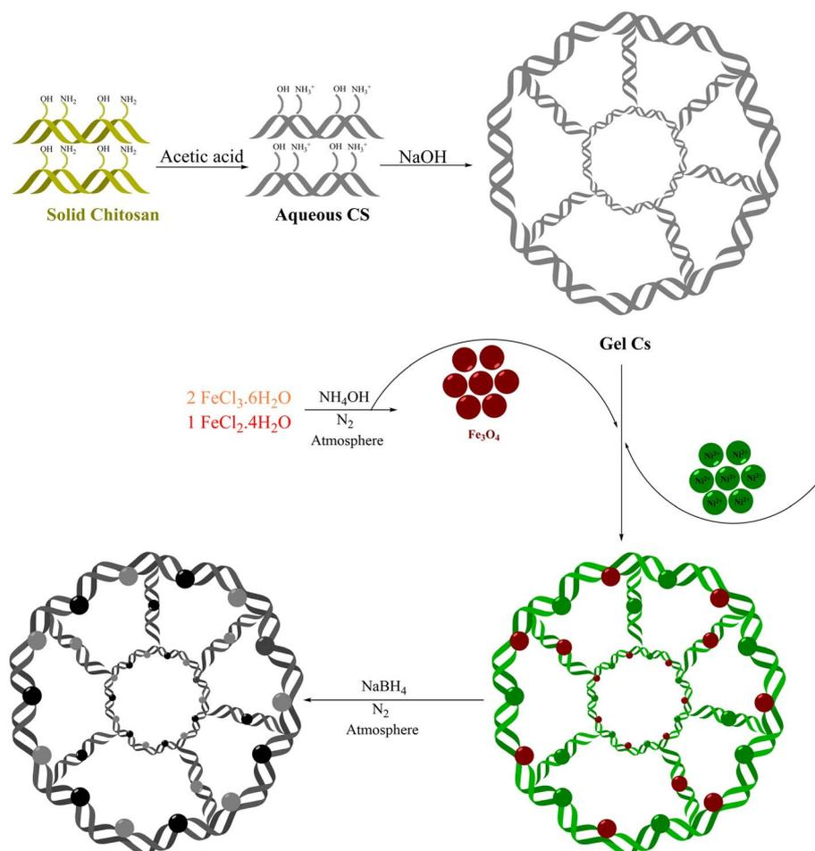
**Scheme 2** Schematic illustration of the preparation of the Fe<sub>3</sub>O<sub>4</sub>@CS@Ni<sub>2</sub>B nanocomposite.
