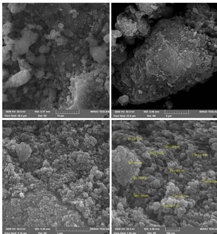
Fig. 8 FESEM image of the  $\text{Fe}_3\text{O}_4@\text{CS@Ni}_2\text{B}$  nanocomposite.
