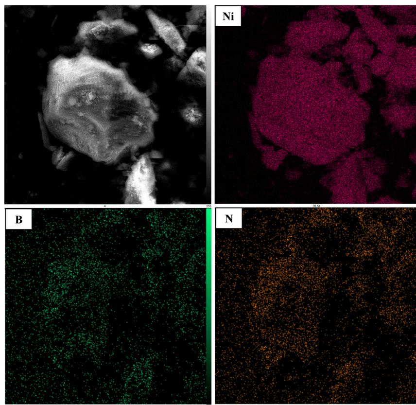
Fig. 9 SEM-based elemental mapping of the as-synthesized  $\text{CS}@\text{Ni}_2\text{B}$  nanocomposite.
