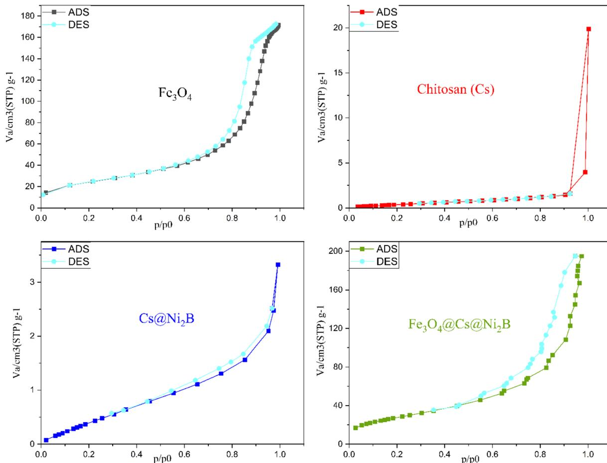
Fig. 5 N<sub>2</sub> adsorption–desorption isotherms of Fe<sub>3</sub>O<sub>4</sub>, chitosan (CS), CS/Ni<sub>2</sub>B and Fe<sub>3</sub>O<sub>4</sub>/CS/Ni<sub>2</sub>B.
