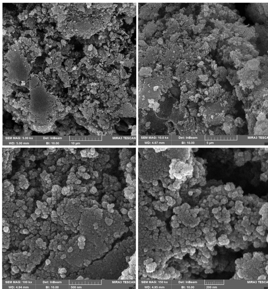
Fig. 14 Reusability FESEM image of the  $\text{Fe}_3\text{O}_4@\text{CS}@\text{Ni}_2\text{B}$  nanocatalyst after 3 runs.
