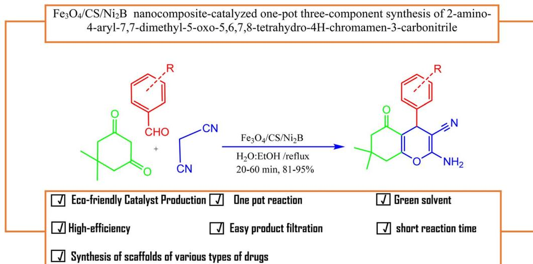
**Scheme 1** Fe<sub>3</sub>O<sub>4</sub>@CS@Ni<sub>2</sub>B nanocomposite-catalyzed one-pot three-component synthesis of 2-amino-4-aryl-7,7-dimethyl-5-oxo-5,6,7,8-tetrahydro-4H-chromamen-3-carbonitrile.
