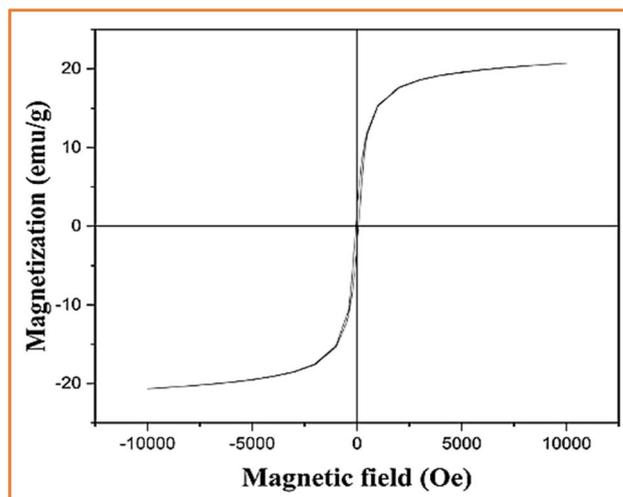
Fig. 11 VSM magnetization diagram of the  $\text{Fe}_3\text{O}_4@\text{CS}@Ni_2B$  nanocomposite.
