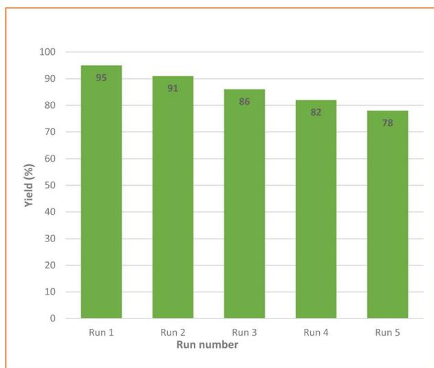
Fig. 12 Reusability diagram of the  $\text{Fe}_3\text{O}_4@\text{CS}@\text{Ni}_2\text{B}$  nanocatalyst.
