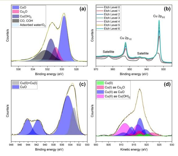
Fig. 6 High resolution XPS spectra of s-Cu(x) prior to ECR studies, showing (a) O 1s, (b) Cu 2p along with a depth profile, (c) Cu 2p<sub>3/2</sub>, and (d) Cu LMM Auger spectral analysis.
