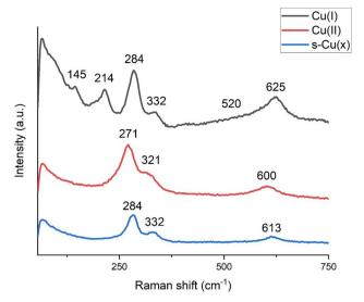
Fig. 5 Raman shift analysis of samples predominantly composed of Cu<sub>2</sub>O, as Cu(ı), CuO, as Cu(ıı), and laser structured Cu with mixed oxidation states, s-Cu(x).
