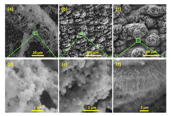
Fig. 3 (a-c) SEM micrographs of femtosecond laser-structured Cu (20  $\mu$ m parallel line spacing), with (d-f) corresponding zoomed-in views. (ad) Cu structured in Ar, showing spherical submicron and nanoparticles. (b-e) Cu structured in air, showing spherical submicron and nanoparticles. (c-f) Cu structured in air and annealed at 350 °C, depicting nanowire-decorated microfeatures.
