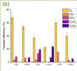
Fig. 8 (a) Faradaic efficiency of s-Cu(x) for  $H_2$  and  $C_{2+}$  gases as a function of vessel pressure. (b) Faradaic efficiency of all gaseous products observed for unstructured and hierarchically structured Cu(0), Cu(x), and Cu(II) electrodes, respectively.
