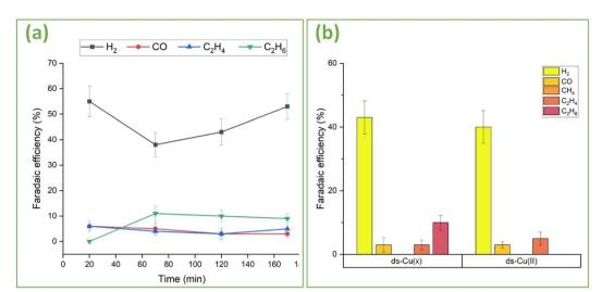
Fig. 9 (a) Faradaic efficiency of ds-Cu(x) for gaseous products as a function of time. (b) Comparison of Faradaic efficiency of ds-Cu(x) and ds-Cu(y) for gas products at 4 bar pressure.
