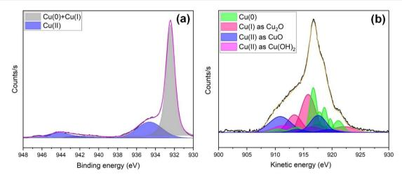
Fig. 7 High-resolution XPS spectra of s-Cu(x) obtained after electrochemical CO<sub>2</sub> reduction, presenting (a) Cu 2p<sub>3/2</sub> and (b) Cu LMM Auger spectral analysis.
