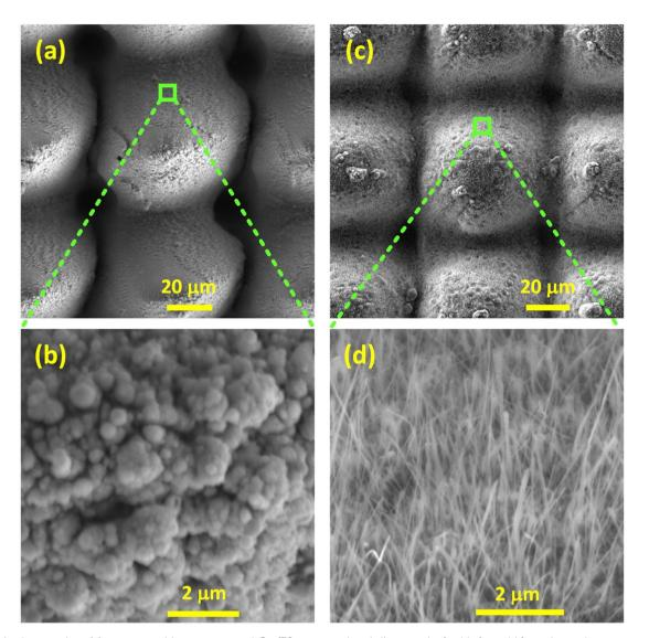
Fig. 4 SEM micrographs of femtosecond laser structured Cu (70  $\mu$ m crosshatch line spacing) with (a and b) no thermal treatment depicting submicron and nanospheres decorating microdomes, and (c and d) thermally treated at 350 °C in air, showing nanowires decorating the microdomes.
