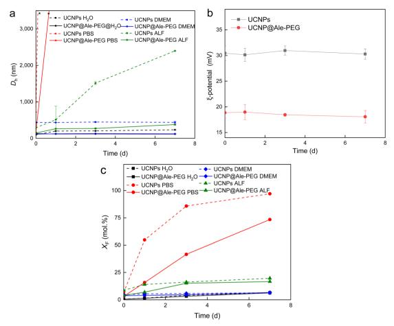
Fig. 5 Time dependencies of (a) hydrodynamic diameter D<sub>h</sub> in water, PBS, DMEM and ALF, (b) ζ-potential of UCNPs and UCNP@Ale-PEG nanoparticles in water and (c)  $F^-$  ion molar fraction ( $X_F$ ) in the supernatants after incubation of particles in water, PBS (pH 7.4), DMEM and ALF at 37 °C. \* Beyond the scope of measurement.
