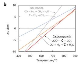
Fig. 4 Effect of reaction temperature on reaction efficiency for CO-CCVD by the seed method using Co SCs. (a) Reaction efficiency of Co catalysts used in the CNT growth reaction at several temperatures in the reaction for 60 min, determined by TG measurements under an air atmosphere. The amount of Co on silica was set to 2 wt% for all catalyst samples. (b) Gibbs free energy of the CO-CCVD reaction, simulated by thermodynamic equilibrium calculation (Gibbs free energy minimization algorithm).
