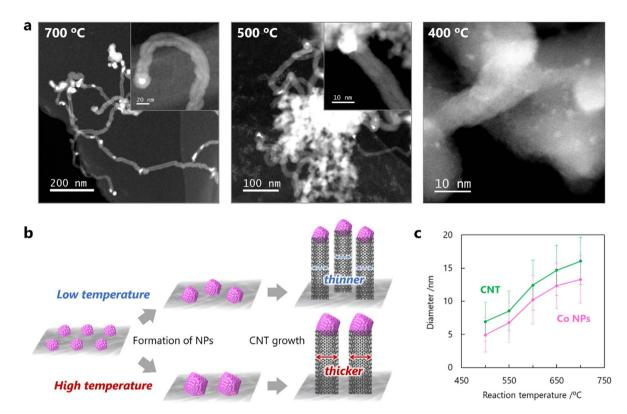
Fig. 3 Effect of reaction temperature on CNT growth by the seed method using Co SCs. (a) High-magnification and low-magnification (inset) STEM images of CNTs grown from Co NPs using a mixture of  $CO/H_2 = 1$  at 700, 500, and 400 °C for 60 min. (b) Proposed scheme of CNT growth by the seed method using Co SCs depending on the reaction temperature. (c) Temperature-dependence of the diameters of Co NPs and grown **CNTs**
