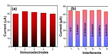
Fig. 8 (a) Repeatability study of five different nano-biochips of BSA/anti-IL8/nano-ceria/ITO; (b) interference study of fabricated BSA/anti-IL8/nano-ceria/ITO electrode with antigen of IL8 and other interferents using the DPV technique.
