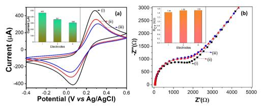
Fig. 4 (a) Cyclic voltammetry studies of (i) nano-ceria/ITO, (ii) anti-IL8/nano-ceria/ITO, (iii) BSA/anti-IL8/nano-ceria/ITO electrodes (b) electrochemical impedance response signal of (i) nano-ceria/ITO, (ii) anti-IL8/nano-ceria/ITO, (iii) BSA/anti-IL8/nano-ceria/ITO electrodes conducted in PBS (pH 7.4) containing  $[Fe(CN)_6]^{3-/4-}$ .
