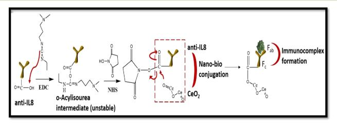
Fig. 7 Mechanism of activation of IL8 antibody using EDC: NHS chemistry, binding with nano-ceria for nano-bio conjugation and attachment of activated antibody with antigen for immunocomplex formation.
