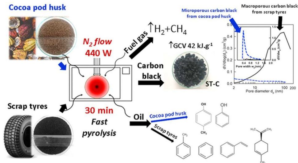
Fig. 5 Illustration of microwave pyrolysis process. Reproduced from ref. 35 with permission from Elsevier, copyright 2025.
