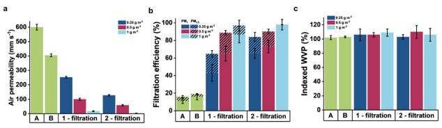
Fig. 4 (a) Air permeability, (b) aerosol particulate filtration efficiency and (c) indexed water vapour transmission rate of uncoated woven fabric (A), ZIFcotton (B) and ZIF-BC coated woven fabric fabricated with the single filtration strategy (1-filtration) and double filtration strategy (2-filtration), while PM<sub>1</sub> and PM<sub>2.5</sub> denote particulate matter with size less than 1 and 2.5 μm respectively.
