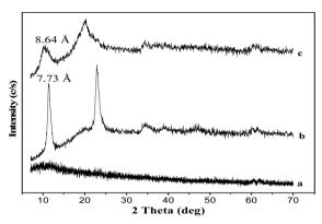
Fig. 3 PXRD of (a) the wet cake obtained using chloride precursor and the vacuum-dried wet cake obtained using (b) chloride and (c) nitrate metal precursor at 100 °C
