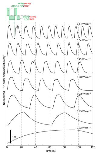
Fig. 6 Multiple cycles of writing and erasing of the thin circular polarization holograms relative to the writing beam intensity at (a) 0.02 W cm $^{-2}$ , (b) 0.13 W cm $^{-2}$ , (c) 0.22 W cm $^{-2}$ , (d) 0.33 W cm $^{-2}$ , (e) 0.45 W cm $^{-2}$ , (f) 0.54 W cm $^{-2}$  and (g) 0.64 W cm $^{-2}$ .
