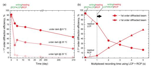
Fig. 5 (a) Retention ratio of -1st order diffraction efficiency for thin circular polarization hologram at various storage conditions. (b) Variation of  $\pm 1$ st order diffraction efficiency with different recording times of the second hologram for polarization hologram multiplexing.
