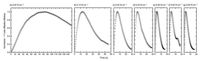
Fig. 4 Time variation of normalized -1st order diffraction efficiency for thin circular polarization hologram relative to the writing beam intensity at (a)  $0.02~{\rm W~cm^{-2}}$ , (b)  $0.13~{\rm W~cm^{-2}}$ , (c)  $0.22~{\rm W~cm^{-2}}$ , (d)  $0.33~{\rm W~cm^{-2}}$ , (e)  $0.45~{\rm W~cm^{-2}}$ , (f)  $0.54~{\rm W~cm^{-2}}$  and (g)  $0.64~{\rm W~cm^{-2}}$
