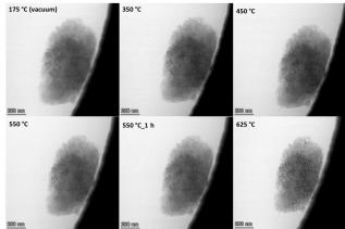
Growth of MnO<sub>x</sub> nano particles in a TEM (200 kV). Temperature from the start of the irradiation is displayed on each image. Diffusion of  $MnO_x$  on the surface is seen. Beam current density: 200 A cm<sup>-2</sup>. Each image represents an area of  $9.2 \times 9.2 \text{ nm}^2$
