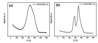
Fig. 10 H<sub>2</sub>-TPR profile of 20Mn/SBA-15 catalyst prepared by (a) dry impregnation, and (b) wet impregnation.
