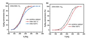
Fig. 13 Thermal stability evaluation of catalyst: (a)  $20 \text{Mn/SBA-15}_{d}$  (b)  $20 \text{Mn/SBA-15}_{w}$ .
