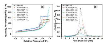
Fig. 4 (a) N<sub>2</sub> adsorption desorption isotherm (b) BJH pore size distribution of prepared catalysts.
