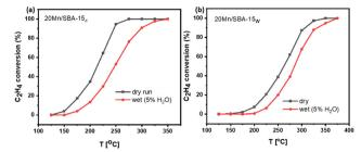
**Fig. 12** Catalytic activity tests of MnO $_{\rm X}$  catalysts at GHSV of 64 000 ml  ${\rm g_{cat}}^{-1}\,{\rm h}^{-1}$  in dry and wet conditions; (a) 20Mn/SBA-15 $_{\rm d}$  and (b) 20Mn/SBA-15 $_{\rm w}$ . Test conducted with 850 ppm ethylene, 15% O $_{\rm 2}$ , 5% H $_{\rm 2}$ O (wet conditions) and balance N $_{\rm 2}$  at 250 °C.
