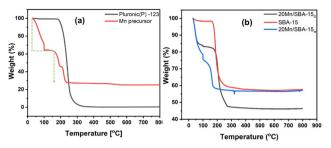
Fig. 3 TGA curves of (a) P-123 template and Mn(NO<sub>3</sub>)<sub>2</sub>·xH<sub>2</sub>O and (b) TEOS condensed on P-123, and 20 wt% Mn loaded on SBA-15 at a heating rate of 10 °C min<sup>-1</sup>
