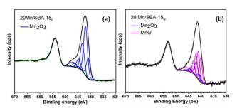
Fig. 9 XPS spectra of Mn 2p of (a) 20Mn/SBA-15<sub>d</sub> and (b) 20Mn/SBA-15<sub>w</sub> catalysts.
