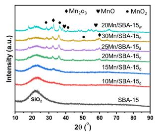
Fig. 1 X-ray diffraction patterns of all the  ${\rm MnO_x/SBA}\mbox{-}15$  prepared catalysts.
