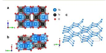
(a) and (b) Monoclinic crystal structure of M-TbTaO<sub>4</sub> (space group 12/a). (c) The distorted diamond lattice of Tb site. The unit cell is shown in thin grey lines.
