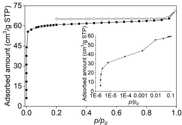
Fig. 4  $N_2$  adsorption (solid symbols)/desorption (open symbols) isotherm at 77 K of the NaX-rich, 3D-printed zeolite-geopolymer composite.
