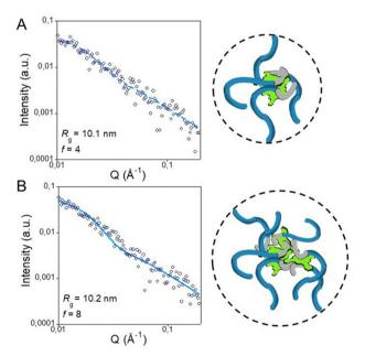
Fig. 5 SAXS results and respective depictions of the morphologies revealed, with form factor in water of SLA-Pc25 (A) and SLA-Pc212 (B). Values of  $R_{\rm q}$  and arm number (f) were obtained through fits of the Dozier star model to the experimental data (continuous lines).
