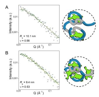
Fig. 3 SAXS results and respective depictions of the morphologies revealed, with form factor in water of  $SCNP-Pc2_5$  (A) and  $SCNP-Pc2_{12}$  (B), Values of  $R_g$  and  $\nu$  were obtained through fits of a generalized Gaussian coil function (continuous lines) to the experimental data.
