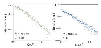
Fig. 2 (A) SAXS results revealing the form factor of  $SCNP-Pc2_0$  in water. Line is a fit of a generalized Gaussian coil function, yielding the values of the  $R_{\rm g}$  and  $\nu$  parameters. (B) SAXS results revealing the form factor of  $SLA-Pc2_0$  in water. Line is a fit of the Dozier star model, yielding the values of the  $R_{\rm g}$  and f parameters.
