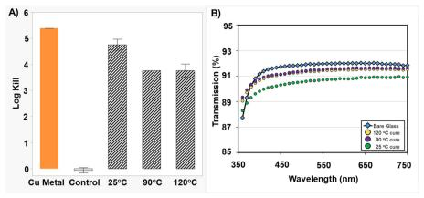
Fig. 7 Antimicrobial efficacy and optical transmission results for Ferro 221 glass coatings dosed with copper glass-ceramic (CGC) powder extracts with triethyl phosphite (TEP) ([Cu]<sub>Tot</sub> = 600 ppm) and cured at different temperatures. A. Average log-kill values against *S. aureus* for various coating cure conditions. Control sample has no antimicrobial additive. Error bars represent the standard deviation of duplicate samples. B. Optical transmission measurements.
