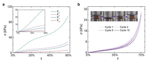
Fig. 4 Mechanical properties *via* compression testing of the biobased self-blown PC foams. (a) Stress-strain ( $\sigma$ - $\varepsilon$ ) curves of foams  $F_1$ - $F_4$  with different biobased polyols. (b)  $\sigma$ - $\varepsilon$  curves of the CNSL-based foam,  $F_2$ , for 10 compression and release cycles up to 70% strain. Inset: photographs of  $F_2$  being subjected to cyclic compression.
