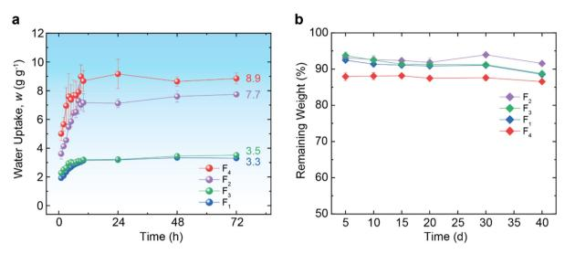
Fig. 3 Water uptake and stability of the biobased self-blown PC foams over time. (a) Maximum ( $w = 8.9 \text{ g g}^{-1}$ ) and minimum ( $w = 3.3 \text{ g g}^{-1}$ ) water uptake within 72 h, depending on the polyols used. (b) *In vitro* degradation behavior of the foams in neutral pH water for 40 days.
