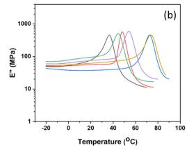
Fig. 4 DMA data showing the storage (a) and loss modulus (b) of the polyesters (1 Hz, 0.1% strain).
