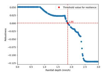
Fig. 10 Robustness of the system under rainfall computed for different rainfall intensities (mm h<sup>-1</sup>). The stressor is applied to the inlet of the system. The resilience (red dot) is the largest rain intensity while still having non-negative robustness. This is equal to 1.86 mm  $h^{-1}$
