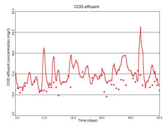
Fig. 11 Effluent concentrations of COD effluent concentration (mg  $\Gamma^{-1}$ ). The continuous red line is the modelled COD effluent concentration and the red diamonds are the measured composite data.
