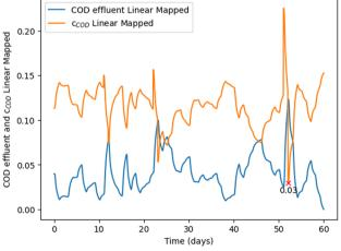
Fig. 5 In both graphs, red "x" denotes the time and the magnitude when the systems was closest to failure. Top. Effluent concentrations (BOD) and robustness ( $c_{BOD}$ ) after linear mapping over a 60 day time horizon. Bottom. Effluent concentrations (COD) and robustness ( $c_{COD}$ ) after linear mapping over a 60 day time horizon.
