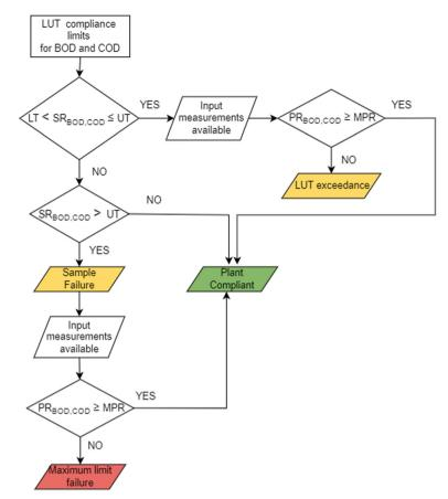
Fig. 2 Subset of the logic diagram for the compliance regulations on WRRFs.
