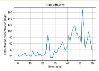
Fig. 12 COD effluent concentration (mg l<sup>-1</sup>) of one of the Monte Carlo simulations in GPS-X.
