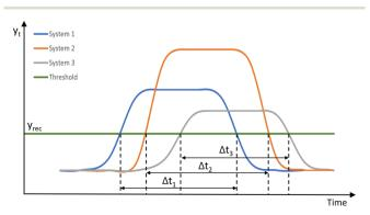
Fig. 9 Recovery behaviours of three systems under stressors. Systems exhibit acceptable recovery behaviours when the times  $\Delta t_1$ ,  $\Delta t_2$ ,  $\Delta t_3 \leq T$ .
