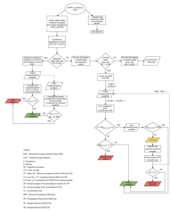
Fig. 1 The logic diagram for the compliance regulations on WRRFs.
