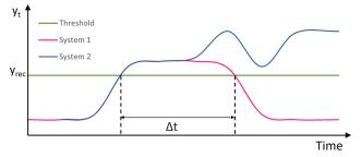
Fig. 8 Examples of responses of two systems under a stressor. System 1 (magenta) is resilient recovering within time  $\Delta t \leq T$ . System 2 (blue) is not resilient as it does not recover at any time.
