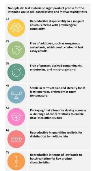
Fig. 1 Target product profile (TPP) of nanoplastic test materials for in vitro and in vivo use.
