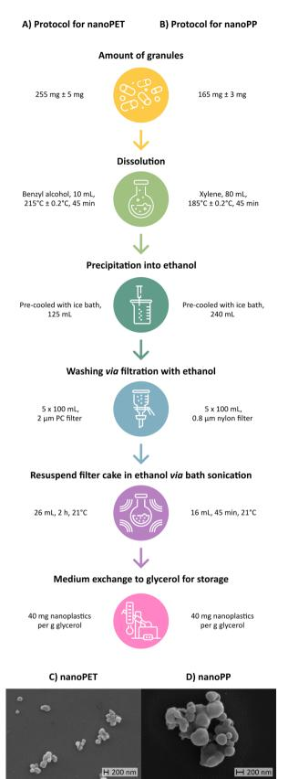
Fig. 2 Production scheme of PET (A) and PP (B) nanoplastic suspensions. Overview of controlled parameters and the experimental settings used. Representative SEM micrographs of PET (C) and PP (D) nanoplastics.
