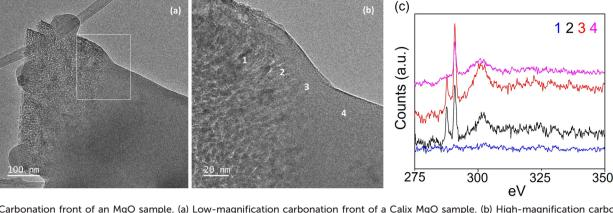
Fig. 7 Carbonation front of an MgO sample. (a) Low-magnification carbonation front of a Calix MgO sample. (b) High-magnification carbonation front of a Calix MgO sample. (c) EELS spectra from the MgO through the carbonation front to the MgCO<sub>3</sub> (1-4).
