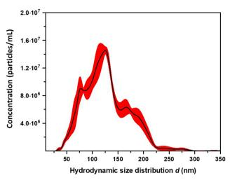
Fig. 2 The total concentration of the nanoparticles produced in the aqueous dispersion and their hydrodynamic size distribution derived from NTA analysis as observed from five consecutive measurements on the same sample, with the black line representing the mean hydrodynamic diameter and the red showing the standard deviation.
