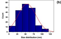
Fig. 1 (a) TEM micrograph of the formed nanoparticles. (b) The size distribution of nanoparticles was calculated from TEM micrographs using ImageJ software on a total of 180 particles.
