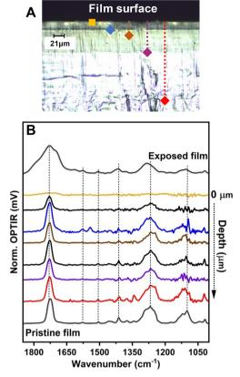
Fig. 2 A) Optical cross-sectional image of the weathered PET film with color-coded markings for spectral acquisition. B) Representative OPTIR spectra collected across the film cross-section. The presented spectra were acquired at the surface (gold), 25  $\mu m$  (blue), 35  $\mu m$ (brown), 85  $\mu m$  (purple), and 215  $\mu m$  (red) from the surface. The black traces were representative spectra collected at intermediate depths between the regions identified with distinct color markings.
