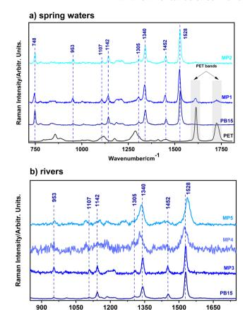
Fig. 6 Typical Raman spectra collected from abundantly observed blue fibers from two spring water sources (a) (Josani and Albioara, Romania) and two rivers (b) (Homorod and Somes, Romania); the spectra of PB15 and PET are given for reference; characteristic bands representing the highest intensity, although broadened, bands of Cuphthalocyanine are observed (785 nm excitation).
