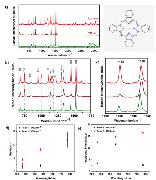
Fig. 2 Raman spectra of the CuPc pigment (the molecular structure is shown in the inset) at three excitation wavelengths, 632.8 nm, 785 nm and 532 nm, in the range of a) 100–3200 cm<sup>-1</sup>, b) 600–1750 cm<sup>-1</sup> and c) 1400–1550 cm<sup>-1</sup>; and the variation of d) FWHM and e) integrated area values for the two highest intensity bands of CuPc, 1452 cm<sup>-1</sup> and 1528 cm<sup>-1</sup>, as a function of excitation wavelength; the error bars indicate standard deviation.
