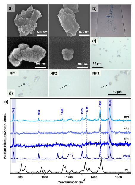
Fig. 8 a) SEM/TEM images of blue nanoplastics resulting from the fragmentation of the PP-BL-003 sample; b) macroscopic and c) optical microscopy images of the blue micro- and nanoplastic particles spread on a microscope slide; d) optical microscopy images of three blue nanoplastics (NP1, NP2 and NP3) and e) their corresponding Raman spectra (excitation: 632.8 nm) together with the spectra of PB15 pigment (excitation: 632.8 nm) and PP (excitation: 785 nm) for reference.
