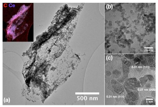
Fig. 3 (a-c) HRTEM images of CeO<sub>2</sub> nanoparticles grown on a GO sheet (CeGO10 sample) with EDS elemental mapping (inset).
