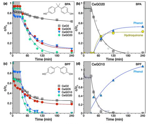
Fig. 7 Kinetics of the photocatalytic decomposition of (a) BPA and (c) BPF on ceria and CeGO composites; (b) kinetics of decomposition of BPA and product formation with the CeGO20 sample and (d) kinetics of decomposition of BPF and product formation with the CeGO10 sample as obtained by HPLC-HRMS analysis of the extracted samples. The shadow points in Fig. 7b and d show the first run of the degradation test analyzed by HPLC-DAD.
