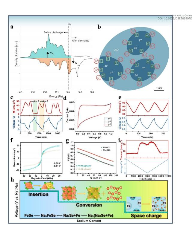
**Fig. 5** Fe<sub>3</sub>O<sub>4</sub>/Li cell's (a) schematic of spin-polarized density of states at the surface of ferromagnetic metal grains (before and after discharge), which is opposite to the bulk spin polarization for the case of Fe. E<sub>F</sub>, Fermi energy. (b) Formation of a space-charge zone in the surface capacitance model for extra lithium storage. Reproduced with permission.<sup>57</sup> Copyright 2021, Nature Publishing Group. (c) Time-sequenced operando
