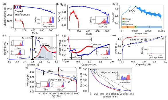
Fig. 2 Feature extraction and divergence distribution between two aging conditions at 1C, 25 °C (blue) and 2C, 0 °C (red): (a) charging time, (b-1) endof-charge voltage (EOCV), (b-2) schematic illustration of EOCV data collecting during charging-discharging cycles, (c) IC curve shift; (d) DV curve shift; geometry pattern of (e) voltage, (f) capacity deviation, and (g) current. V<sub>1</sub> and V<sub>1</sub>, indicate the charging range within which features are extracted.
