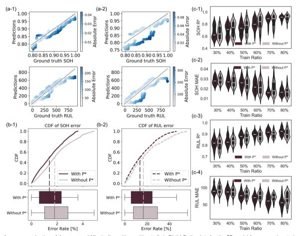
Fig. 4 Performance evaluation of the proposed ML pipeline with or without all six P\*. (a) Parity plots for the RF model for one random train-test split (80% training, 20% testing): (a-1) with P\* and (a-2) without P\*. (b) Cumulative error distributions comparing predictions with and without P\* for both (b-1) SOH and (b-2) RUL. (c) Monte Carlo simulations of model with 100 random seeds, using varying train-test ratios, with and without P\*
