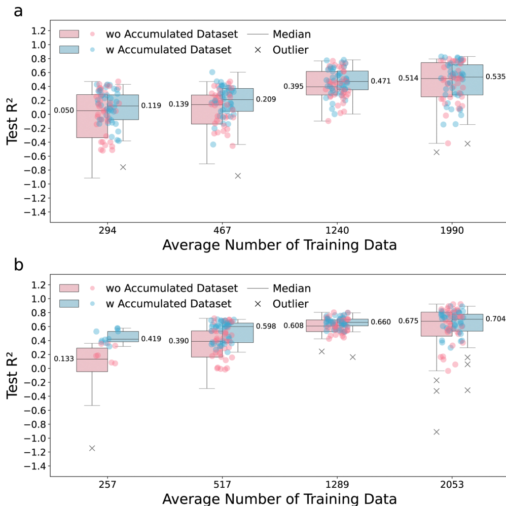
Fig. 5 Test R^2 performance across training dataset sizes without or with the accumulated dataset for two ternary systems. Box plots illustrating test R^2 for two material systems: (a) PM6:Y6:IT-4F and (b) PM6:D18:L8-BO, in relation to the average number of pieces of training data, corresponding to about 10, 20, 50 and 80% without and with the accumulated dataset (PM6:L8-BO material system composed of 20 199 data points). Each data point for the R^2 is represented as a circle-shaped marker. Pink and blue boxes represent the interquartile range (IQR) of the test R^2 without and with the accumulated data, respectively, extending from the first quartile (Q1) to the third quartile (Q3). Each median is indicated by a solid line within the box, accompanied by a numerical value. The boundaries of the whiskers follow the 1.5 IQR rule to identify outliers, where the lower whisker extends to the lowest data point above Q1 - 1.5 \times (Q3 - Q1) , and the upper whisker extends to the highest data point below Q3 + 1.5 \times (Q3 - Q1) . Outliers are denoted by a marker 'x'.
