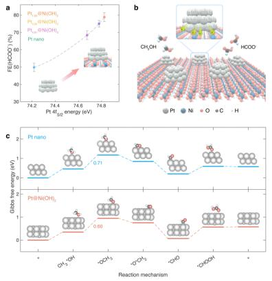
Fig. 4 Methanol e-refinery mechanisms towards formate. (a) The relationship between Pt  $4f_{5/2}$  energy and formate faradaic efficiencies of  $Pt_x@Ni(OH)_2$  (x = 1.05, 3.00, and 4.91) and Pt nano. (b) The reaction diagram of methanol e-refinery on Pt-loaded Ni(OH)<sub>2</sub>. (c) Possible reaction route and the corresponding computed free energy changes of methanol e-refinery towards formate on Pt and Pt-loaded Ni(OH)<sub>2</sub>.
