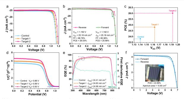
Fig. 4 (a) J-V curves of the control, target-1 and target-2 devices under reverse scan. (b) J-V curves of reverse and forward scans for the optimized target-2 device. (c) PCE and  $V_{oc}$  of the control, target-1 and target-2 devices. (d) Mott-Schottky plots for the corresponding devices. (e) EQE spectra of the corresponding devices. (f) J-V curves of reverse and forward scans for the target-2 film based mini-module (10.80 cm<sup>2</sup>).
