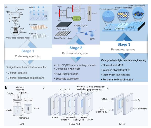
Fig. 2 (a) Development progress of the acidic CO<sub>2</sub>RR.<sup>26,64</sup> Reproduced with permission from ref. 26. Copyright 2002, Elsevier. Schematic configuration of CO<sub>2</sub>RR electrolyser development: (b) H-cell, (c) flow cell, and (d) MEA.
