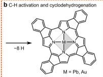
Fig. 1 (a) Reversible on-surface metalation of H<sub>2</sub>(TPP). Reaction with Pb at 300 K yields Pb(TPP), which undergoes demetalation at elevated temperatures. (b) Thermal C-H activation and (cyclo)dehydrogenation. Only one possible product is shown. The released H atoms engage in the demetalation of Pb(TPP) as shown in (a)
