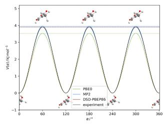
Fig. 3 Relaxed surface scan with respect to the methyl torsional angle  $\alpha$  in kJ mol<sup>-1</sup> for the experiment compared to the predictions by the PBEO/, MP2/ and DSD-PBEP86/aVTZ levels of theory.
