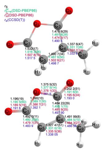
Fig. 9 Comparison of the bond distances of itaconic anhydride (top) and citraconic anhydride (bottom) from Kraitchman's substitution structure (black), a semi experimental equilibrium structure (green) as well as mass dependent  $r_m^{(2)}$  (red) using DSD-PBEP86 and an equilibrium structure at the CCSD(T) level of theory (purple). All values are given in Å.
