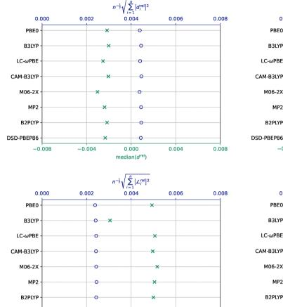
Fig. 7 Comparison of standard and median deviations of bond lengths  $d^{\rm rel}$  (above) and angles  $\angle$  rel (below) from CCSD(T) for all  $r_m$  structures in citraconic anhydride (8 and 11 data points).
