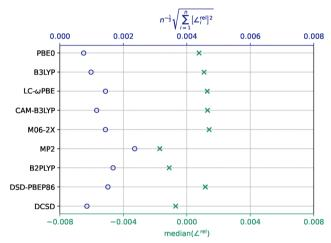
Fig. 6 Comparison of standard and median deviations of bond lengths  $d^{\text{rel}}$  (above) and angles  $\angle$  rel (below) from CCSD(T) for all  $r_{0\rightarrow e}^{\text{SE}}$  structures in itaconic anhydride (4 and 4 data points)
