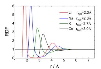
**Fig. 6** Radial distribution functions, RDF(r), as a function of the distance between the oxygen for Li, Na, K and Cs in water. The data points were scanned by hand from Fig. 4a of Singh  $et\ al.$  For large radii, the scanned function was smoothed with an exponential tail to estimate the mean radius of hydration. For further information see ESI,† Section S4.
