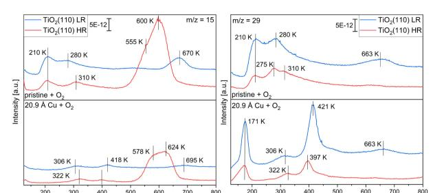
Fig. 5 TPR spectra of a monolayer methanol adsorbed at T = 115 K and methanol with 56 L of oxygen pre-adsorbed at the pristine slightly (LR) and highly (HR) reduced TiO<sub>2</sub>(110) single crystals (top spectra) and 20.9 Å of copper deposited onto the slightly and highly reduced single crystals (bottom spectra). Displayed are the m/z = 15 and m/z = 29 signals for the experiments reaching 800 K at a rate of 2 K s<sup>-1</sup>.
