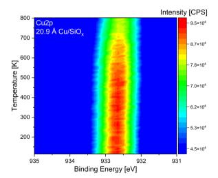
Fig. 1 Temperature-programmed X-ray photoelectron Cu 2p<sub>3/2</sub> spectra after depositing 20.9 Å of copper onto a silicon wafer with a native oxide film. The sample was first cooled down to 120 K and then slowly heated to 800 K with a heating rate of 0.5 K s $^{-1}$  while XP-spectra were recorded. All spectra loops were measured with a pass energy of 30, a step size of 0.15 eV and a dwell time of 25 ms
