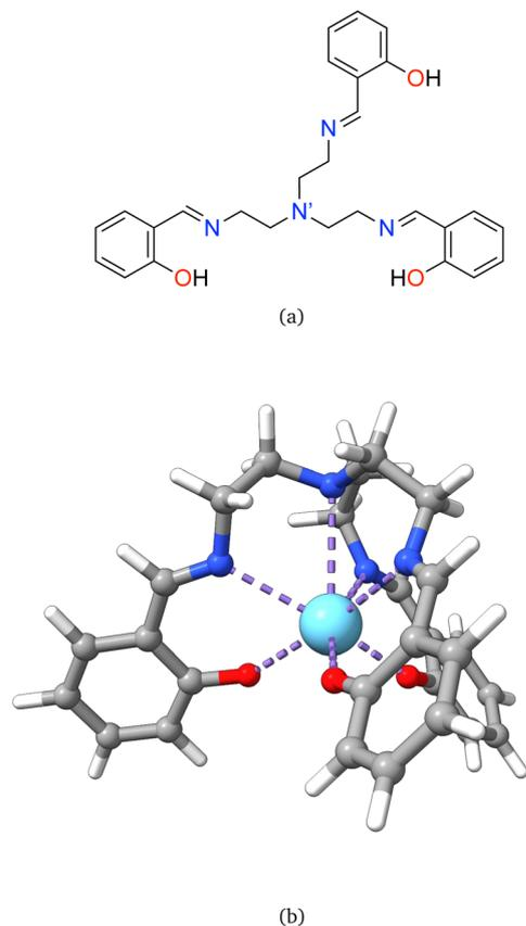
**Fig. 1** (a) Schematic 2D representation of the neutral form of the unbound trensal ligand ( $H_3$  trensal), and (b) the 3D visualization of trensal bound to a trivalent lanthanide ion (oxygen, nitrogen, lanthanide, carbon, and hydrogen are depicted in red, blue, light blue, grey, and white, respectively).
