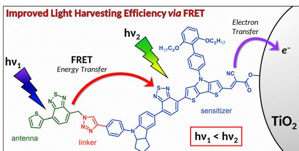
**Improved light harvesting via energy transfer within a benzothiadiazole-based antenna–sensitizer dyad for dye-sensitized solar cells**
