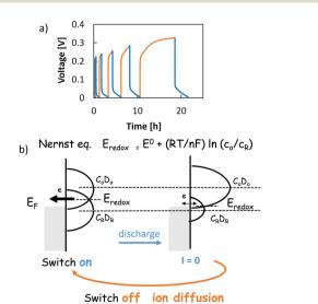
Fig. 6 Voltage behaviour of n-Si/Ge/copper ionic electrolyte/FTO at 80 °C, 100 nA discharge and recovery (a); 45 conceptual diagram of Nernst's equation (b); blue: discharge (switch on), orange: recovery (switch off).  $E_{\rm F}$ : Fermi level.  $E_{\rm O}$ : standard redox potential.  $c_{\rm o}$ ,  $c_{\rm R}$ : concentration of oxidized and reduced elements. Do, DR: density of states of oxidized and reduced ions (Copyright © 2019 Royal Society of Chemistry)
