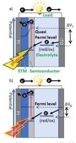
Fig. 5 Schematic image of the output potential by (a) photoexcitation and (b) thermal excitation. ETM: electron transport material<sup>43</sup> (Copyright © 2020 The Chemical Society of Japan).
