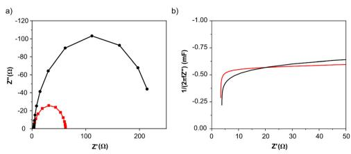
Fig. 4 Electrochemical impedance spectroscopy (EIS) of PdAu/C (red curves) and Pd/C (black curves) in KOH 2 M at 0.4 V vs. RHE: (a) Nyquist plot and (b) capacitance plot.
