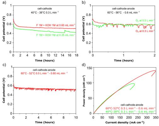
Fig. 6 DFFC stability experiments carried out a single pass fuel feed (galvanostatic – 0.05 A cm<sup>-2</sup>). (a) Variable anode flow; (b) variable cathode flow; (c) high anode and high cathode flow test showing stable power density delivery; (d) power density vs. current density curves at variable cell temperature. All experiments fuel composition 1 M KOH and 1 M HCOOK.
