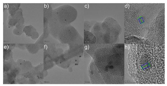
Fig. 1 HR-TEM images of (a)-(c) Pd/C and (e)-(g) PdAu/C and measured lattice spacings of an individual Pd NP (d) and an individual PdAu NP (h).
