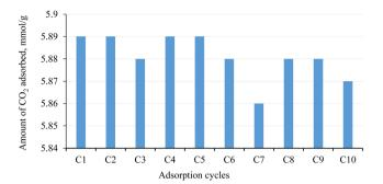
Multi-cyclic CO<sub>2</sub> adsorption performance of L N-K at 0 °C.
