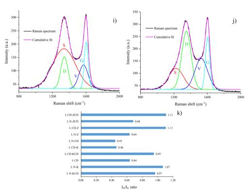
Fig. 3 Curve fitting of Raman spectra (a) L N-K, (b) L CD-K, (c) L N-CD, (d) L CD, (e) L N-KCD, (f) L CD-KCD, (g) L N-Z, (h) L CD-Z, (i) L N-ZCD, (j) L CD-ZCD, and (k)  $I_D/I_G$  ratio.
