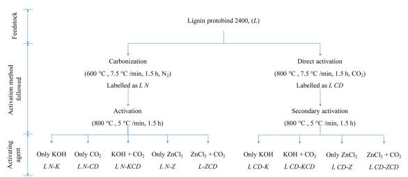
Fig. 1 Methodology followed during the synthesis of activated porous carbon. (L X-Y, where X represents gas purged during carbonization and Y denotes activating agent used; X = N indicates  $N_2$  purging, X = CD indicates  $CO_2$  purging; Y = K denotes KOH activation, Y = CD denotes  $CO_2$  activation).
