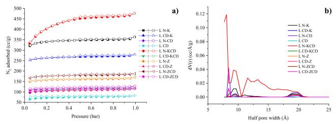
Fig. 4 (a)  $N_2$  adsorption/desorption isotherms of lignin-based activated porous carbons at -196 °C (solid symbols represent adsorption and hollow symbols indicate desorption), and (b) pore size distribution from the NLDFT method using  $N_2$  isotherms at -196 °C.
