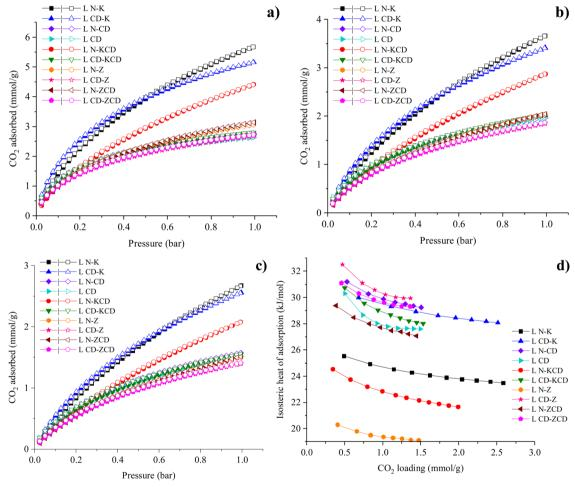
Fig. 5 CO<sub>2</sub> adsorption isotherms at (a) 0 °C, (b) 25 °C, and (c) 40 °C (solid symbols represent adsorption, and hollow symbols indicate desorption), and (d) isosteric heat of CO<sub>2</sub> adsorption.
