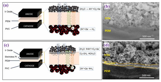
Fig. 12 (a) and (b) represent a schematic view of commercial CCM-electrolyser and SEM image, respectively; (c) and (d) schematic view of modified CCM-electrolyser and its corresponding SEM image. Reproduced with the permission from ref. 111. Copyright 2024, Elsevier.
