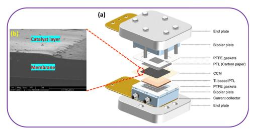
Fig. 2 (a) Schematic look of the PEM water electrolyser components and (b) zoomed view of CCM. Reproduced with permission from ref. 54 and 37. Copyright 2021, ACS and copyright 2010, Elsevier.
