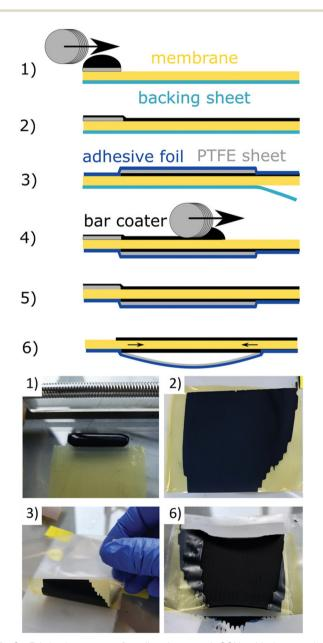
Fig. 9 Fabrication steps of a directly coated CCM with bar coating method. (1), (2) use of the first catalyst layer; (3) use of a protective PTFE layer (grey) with an overlapping adhesive film (blue); (4), (5) use of the second catalyst layer Mayer-rod; (6) the PTFE layer creates gentle tension during drying/shrinking of the CL which protects the CCM from wrinkling. Reproduced with the permission from ref. 97. Copyright 2023, John Wiley and Sons.
