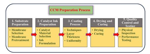
Fig. 3 Schematic sketch of the CCM preparation process.
