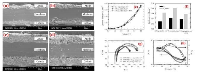
Fig. 7 Cross-sectional SEM pictures of the CCMs before (a), (c) and after (b), (d) AEMWE performance; (e) polarization curves of AEMWE with various membranes; (f) values of R<sub>s</sub> and R<sub>p</sub>; (g) EIS; and (h) Bode plot. Reproduced with the permission from ref. 90. Copyright 2019, Elsevier.
