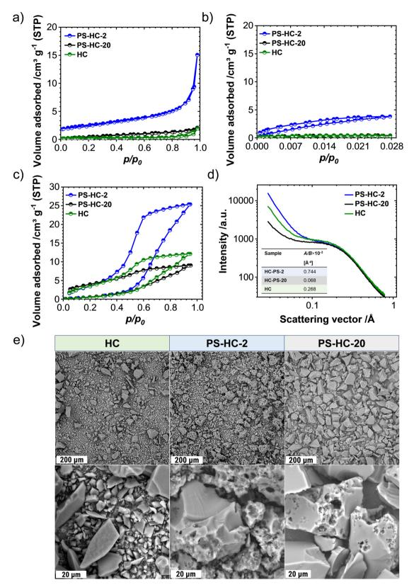
Fig. 2 (a) N<sub>2</sub>-physisorption isotherms at 77 K. (b) CO<sub>2</sub>-physisorption isotherms at 273 K. (c) H<sub>2</sub>O-vapour physisorption isotherms at 298 K. (d) Smallangle scattering curves. (e) SEM images of hard carbon materials.
