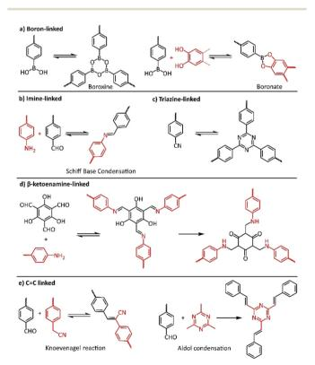
Fig. 3 Typical covalent linkage reactions for COF synthesis
