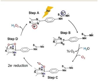
Fig. 13 Mechanism for photocatalytic H<sub>2</sub>O<sub>2</sub> production on the surface of Bpt-CTF. Adapted with permission from ref. 145. Copyright 2022 Wiley.
