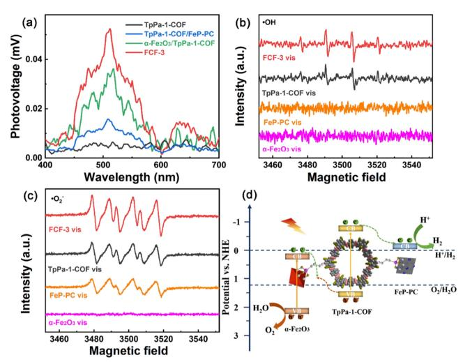
Fig. 11 (a) Surface photovoltage spectra of TpPa-1-COF, α-Fe<sub>2</sub>O<sub>3</sub>/TpPa-1-COF, TpPa-1-COF, TpPa-1-CO EPR spectra of  $\alpha$ -Fe<sub>2</sub>O<sub>3</sub>, FeP-PC, TpPa-1-COF and FCF-3. (d) Proposed mechanistic scheme of redox reactions in the hybrid. Adapted with permission from ref. 129. Copyright 2022 Elsevier.
