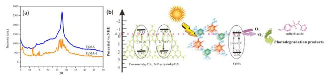
Fig. 17 (a) XRD spectra of the ball-milled material (TpMA) and the solvothermally prepared one (TpMA-1). (b) Band structures of commercial g-C<sub>3</sub>N<sub>4</sub>, self-prepared g-C<sub>3</sub>N<sub>4</sub> and TpMA, and the mechanism of photo-degradation of sulfathiazole catalysed by TpMA. Adapted with permission from ref. 186. Copyright 2021 Elsevier.
