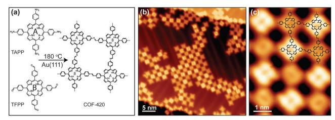
Fig. 5 (a) Schematic representation of the synthesis of COF-420 from the molecular precursors TAPP and TFPP. (b) Representative large-scale STM topographic image of COF-420 on Au(111) (sample bias  $V_s = 0.8 \text{ V}$ , tunnel current  $I_t = 10 \text{ pA}$ ). (c) Close-up STM image of COF-420 with the chemical structure overlaid in the top-right corner ( $V_s = 0.8 \text{ V}$ ,  $I_t = 10 \text{ pA}$ ). Adapted with permission from ref. 94. Copyright 2019 Wiley.
