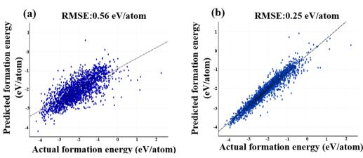
Fig. 8 Visualization of CNN-based model predictions, showcasing the relationship between actual and predicted values using two distinct featurization methods: (a) XRD patterns, and (b) magpie descriptors. As evident from Fig. 8(b), the magpie descriptors resulted in predictions that exhibited sparser and less pronounced deviations from the actual values, in contrast to the other featurization method
