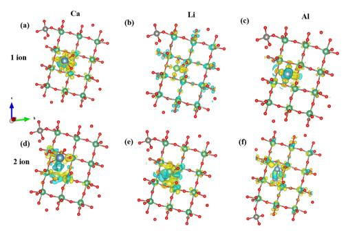
Fig. 7 Charge density plot of the NTO structure for Ca, Li, and Al ions: (a) – (c) depict the scenario with 1 Ca/Li/Al insertion, (d) – (f) illustrate the scenario with 2 Ca/Li/Al insertions. The isosurface level is set at 0.0088 e Å<sup>-3</sup>. The yellow and cyan colors represent charge accumulation and charge depletion, respectively.
