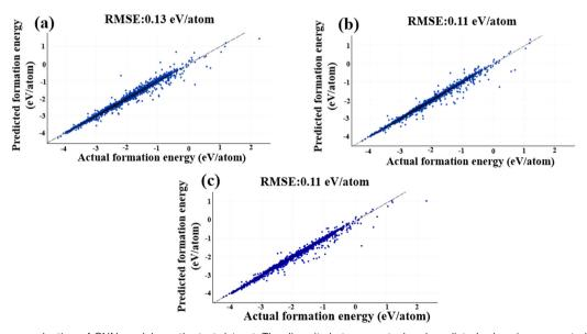
Fig. 9 Performance evaluation of GNN models on the test dataset. The disparity between actual and predicted values is represented through scatter plots and trendlines for (a) MEGNet model, (b) DeeperGATGNN model, and (c) ALIGNN model. Notably, both the ALIGNN and DeeperGATGNN models outperform the human-crafted descriptors and the MEGNet model
