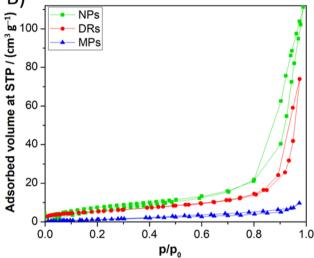
Fig. 1 (A) XRD pattern of the different ZnO microstructures: DRs (red line), MPs (blue line), and NPs (green line). (B) Nitrogen adsorption-desorption isotherms of different ZnO morphologies in powder form.
