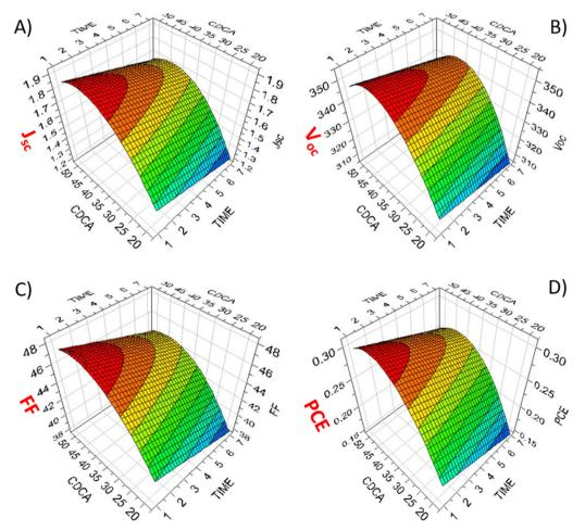
Fig. 4 Isoresponse surfaces show the effect of dye loading time (label: TIME) and CDCA: dye molar ratio (label: CDCA) on the photovoltaic parameters of aqueous DSSCs: (A)  $J_{\rm sc}$ , (B)  $V_{\rm oc}$ , (C) FF, (D) PCE.
