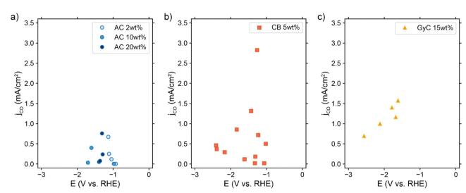
Fig. 8 Resulting partial CO current densities in (a) AC, (b) CB, and (c) GyC suspensions in 0.5 M KHCO<sub>3</sub>, in which  $\frac{1}{3}$  of the solid content consisted of Ag NPs. The cell setup contained 3 mm thick flow channels, separated by a Selemion anion exchange membrane. In each experiment, a graphite or glassy carbon plate current collector was used, and the liquid flow rate was varied between 9 and 18 mm s<sup>-1</sup> (see Table S4 for additional experimental conditions, ESI†).
