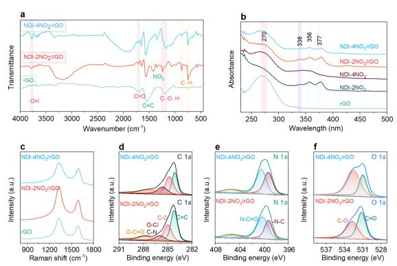
Fig. 2 Structural characterization of the composite materials using spectroscopic and X-ray techniques. (a) Comparative FT-IR spectra of rGO, NDI-4NO2/rGO, and NDI-2NO2/rGO; and (b) UV-vis spectra of different samples. (c) Stacked Raman spectra of rGO, NDI-2NO2/rGO, and NDI-4NO2/rGO, showing the presence of D and G bands. Comparative high-resolution XPS spectra for NDI-2NO<sub>2</sub>/rGO and NDI-4NO<sub>2</sub>/rGO of the (d) C 1s region, (e) N 1s region, and (f) O 1s region.
