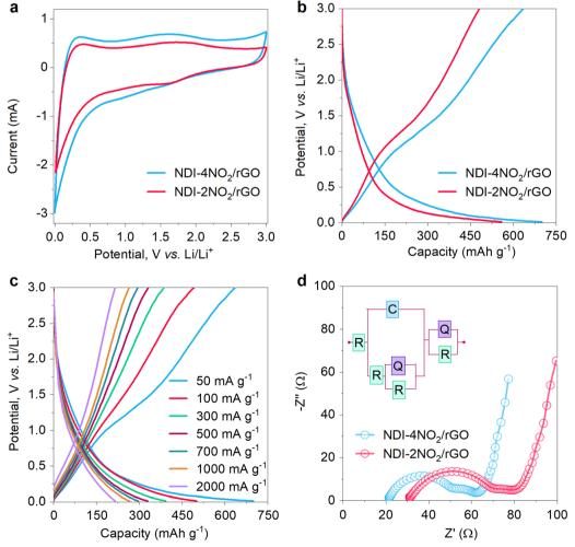
Fig. 3 Electrochemical data for LIB half-cell studies. (a) Comparative CV for the NDI-2NO<sub>2</sub>/rGO and NDI-4NO<sub>2</sub>/rGO samples. (b) The first chargedischarge curve profile at a current density of 50 mA h g<sup>-1</sup> for both samples, (c) the charge-discharge curves of the NDI-4NO<sub>2</sub>/rGO sample at current densities varying from 50 to 2000 mA h  $\rm g^{-1}$ . (d) The comparative Nyquist plots for the NDI-2NO<sub>2</sub>/rGO and NDI-4NO<sub>2</sub>/rGO samples.
