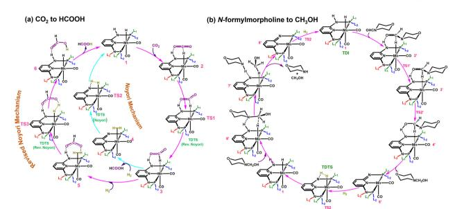
Scheme 1 Possible CO<sub>2</sub> hydrogenation mechanisms to (a) produce HCOOH and (b) the hydrogenation of N-formylmorpholine to CH<sub>2</sub>OH with an aromatic Mn-PNP based catalyst
