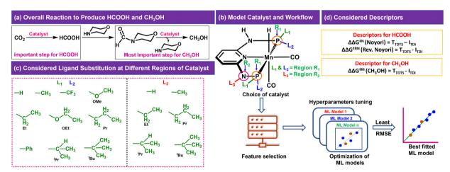
Fig. 1 (a) CO2 reduction reaction steps, (b) model catalyst showing different regions of ligand substitution and general workflow of the work, (c) considered ligands for different regions and (d) suitable descriptors for the reactions.
