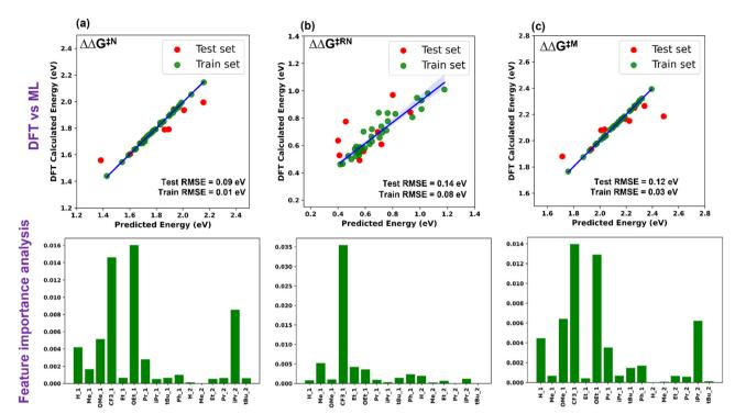
Plot of DFT calculated vs. ML predicted  $\Delta\Delta G^{\ddagger}$  and feature importance for (a) Noyori, (b) revised Noyori and (c) CH<sub>3</sub>OH formation mechanisms.
