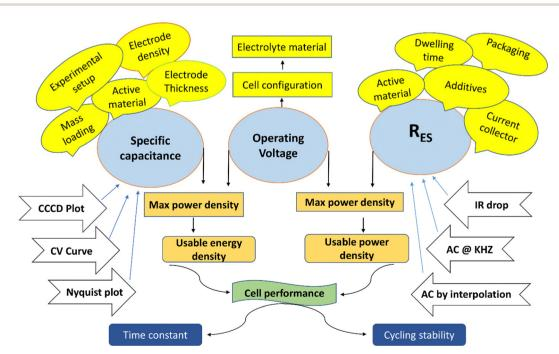
Fig. 4 Schematic showing the significant performance measures, testing methods, and influencing aspects for the evaluation of SCs.
