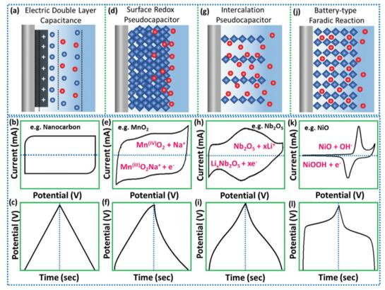
Fig. 3 Electrochemical signatures of energy-storage techniques are shown schematically, together with their representative CV and CD curve shapes: (a) – (c) EDLC, (d) – (f) surface oxidation reduction capacitance, (g) – (i) capacitance intercalation, and (j) – (l) faradaic battery-type. Reprinted with permission from ref. 25. Copyright John Wiley and Sons, 2020
