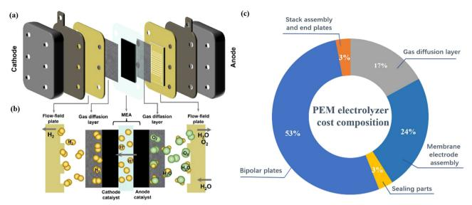
Fig. 1 (a) Schematic illustration and (b) the working principle of PEM water electrolysis. Reproduced with permission from ref. 12. Copyright 2022, Tsinghua University Press. (c) The cost components of a PEM water electrolyzer.
