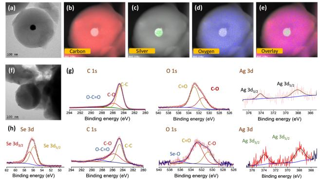
(a) TEM image and (b)-(e) elemental mapping of Ag@CS. (f) TEM image of CS. Deconvoluted XPS spectra (C 1s, O 1s, Ag 3d, Se 3d peaks) of Ag/CS (g) before and (h) after selenisation.
